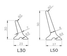
The Extrudingskill Cleats cross cleats, easily weldable on PVC or PU based belts, to transport products on horizontal, vertical and inclined conveyors. They grant a perfect flexibility and resistance to abrasion and oils.
